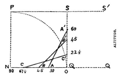
G.M.'s diagram to show the sun's apparent altitude at different latitudes
