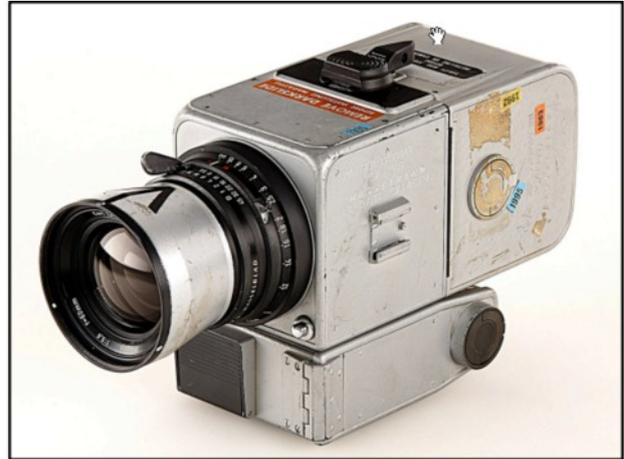
**‘Aperture and Shutter speed locked together’**- The shutter speed and aperture are not fixed together, They have just attached a larger knob to make it easier to use it with gloves. Pushing the knob towards the camera body decouples the aperture and shutter speed rings, and you can turn them separately. That works exactly the same way on similar Hasselblad cameras.
