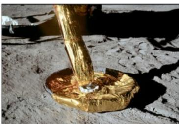
NASA's explanation: 'IN A NUTSHELL: It was blasted away. Dust moved by a rocket exhaust in an airless environment such as the Moon doesn't billow up around the spacecraft and then settle on it: it travels in straight lines away from the vehicle, unhindered by any air resistance, and therefore is unlikely to end up on the vehicle's footpads.'
