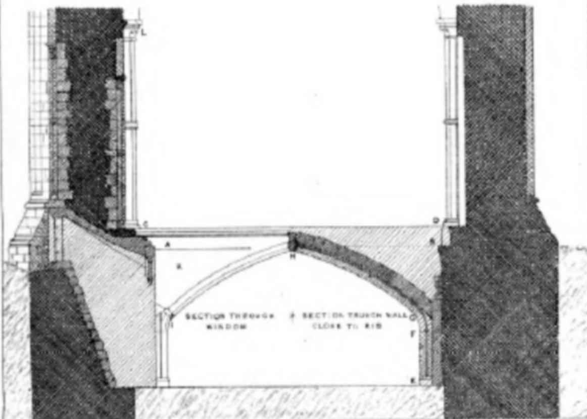
FIG. 6. TRANSVERSE SECTION OF THE WESTERN CRYPT
