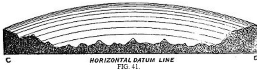
The length of the cable which was laid in 1866, notwithstanding the known irregularities of the bed of the Ocean, would be less than the distance sailed by the paying-out vessel, the "Great Eastern;" whereas, according to the published report, the distance run by the steamer was 1665 miles, while the length of cable payed out was 1852 miles.
