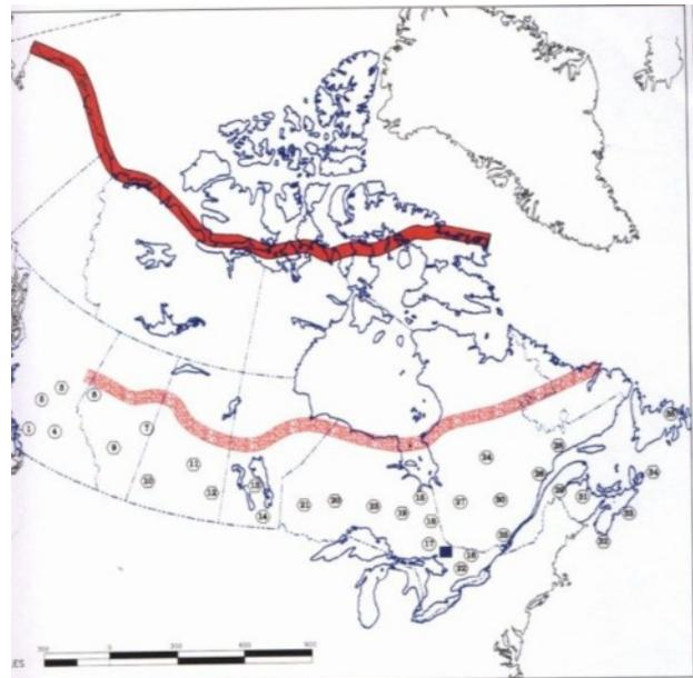
The Mid-Canada Line, extending 2,700 miles from Hopedale, Labrador to Dawson Creek, British Columbia, consisted of 98 powerful Doppler radars 30 miles apart and roughly 300 miles north of the Pinetree Line. Construction of the first station began on October 1, 1956, and the completed system was dedicated on January 1, 1958.
