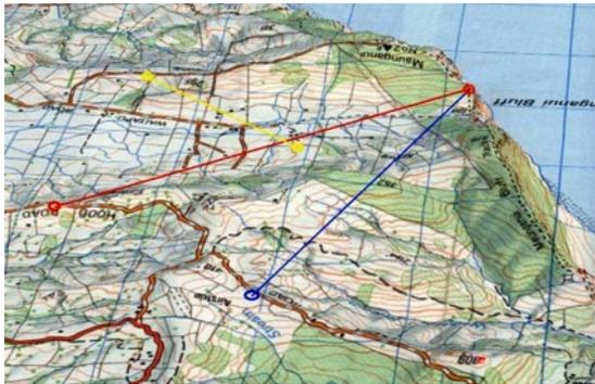
**Figure 11: The blue line runs accurately for 12235 feet from the Benchmark Cleft to a boulder cairn on the hill above the Kerr Road Observatory site.**
