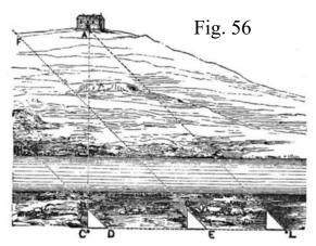
Let A be an object, the distance of which is desired, on the opposite side of a river. Place a rod vertically at the point C, and take a piece of strong cardboard, in the shape of a right-angled triangle, as B, C, D. It is evident that placing the p. 100
