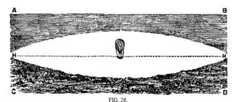
The surface of the earth C, D, appears to rise up to the level of the observer in the car of the balloon; and at the same time, the sky A, B, seems to descend and to meet the earth at the horizon H, H.
