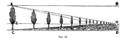
A very good illustration of the difference is given in fig. 76. False or prevailing perspective would bring the lines A, B, and C, D, to the same point H; but the true or natural perspective brings the line A, B, to the point W, because there and there only does A, W, E, become the same angle as C, H, E. It must be the same angle or it is not the vanishing point.
