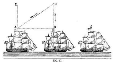
But because the two motions act conjointly, the ball will take the diagonal direction, A, D. By the time the ball has arrived at D, the ship will have reached the position, 13; and now, as the two forces will have been expended, the ball will begin to fall, by the force of gravity alone, in the vertical direction, D, B, H; but during its fall towards H, the ship will have passed on to the position S, leaving the ball at H, a given distance behind it.
