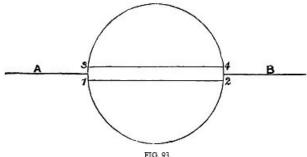
Instead of the line going uninterruptedly through the lens in the direction A, B, it will diverge, and appear at 1, 2; or it will appear above the line A, B, as at 3, 4, if the lens is held to the slightest amount above or below the actual centre.
