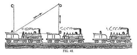
The same result will be observed on throwing a ball upwards from a railway carriage, when in rapid motion, as shown in the following diagram, fig. 48. While the carriage or tender passes from A to B, the ball thrown upwards, from A towards (2, will reach the position D; but during the time of its fall from D to B, the carriage will have advanced to S, leaving the ball behind at B, as in the case of the ship in the last experiment.
