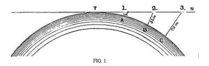
Let the distance from T to figure 1 represent 1 mile, and the fall from 1 to A, 8 inches; then the fall from 2 to B will be 32 inches, and from 3 to C, 72 inches. In every mile after the first, the curvature downwards from the point T increases as the square of the distance multiplied by 8 inches. The rule, however, requires to be modified after the first thousand miles. 1 The following table will show at a glance the amount of curvature, in round numbers, in different distances up to 100 miles.
