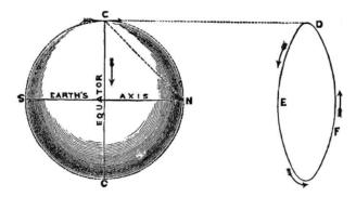
Let C, fig. 87, represent a dipping needle on the "equator" of a globe. A mere inspection of the diagram is sufficient to make it demonstrated that the needle C cannot be horizontal, and at the same time pointing towards the north pole N. If a ship sailed east or west on the equator where the compass is horizontal, it is evident that its north or south end would describe a circle in the heavens equal in magnitude to the circumference of the earth at the equator--as shown by D, E, F.
