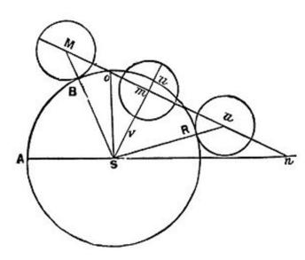
Let A, B, R, (in the following diagram) be a section of the earth's shadow at the distance of the moon; S, n, the path described by its centre, S, on the ecliptic; M, n, the relative orbit of the moon; M, n, S, n, being considered straight lines. Draw S, o, perpendicular to S, n, and S, m, to M, n; the no, and m, are in the places, with respect to S, of the moon in opposition, and at the middle of the eclipse.
