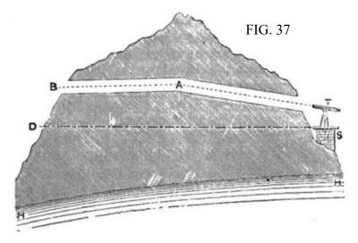
would be 52 feet higher above the sea at H, than it is known to be; because taking D, S, as a tangent, and the length of the tunnel being 8 miles-82 miles x 8 inches = 52 feet.
