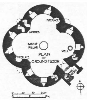
Above right - a plan in section view showing the design of the of the Clifford Tower of likeness to a key handle.
